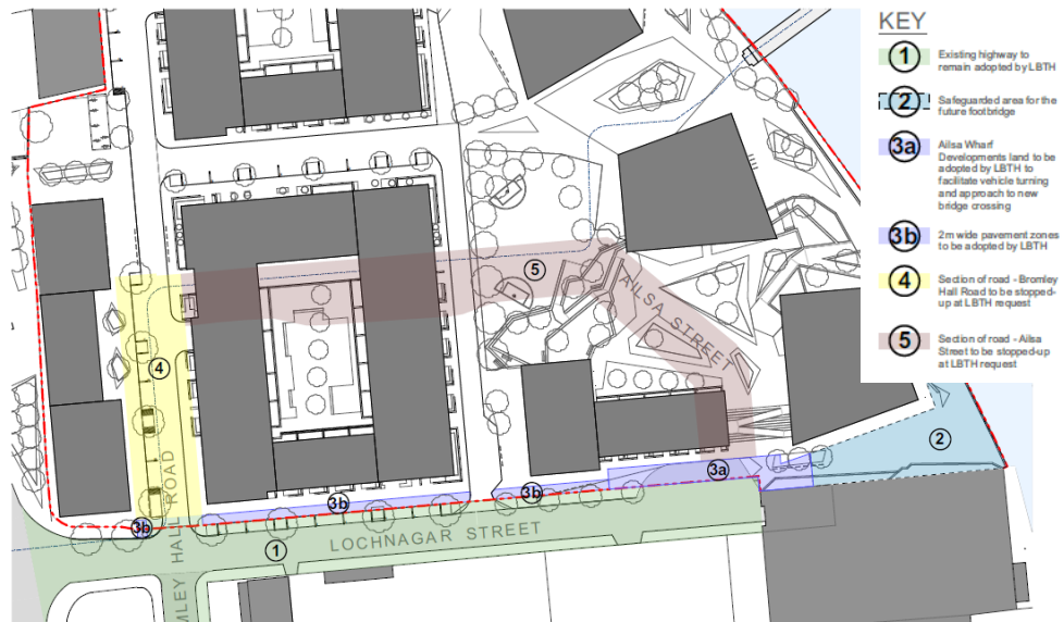
Figure 18- Plan showing highways to be adopted/ stopped up and safeguarded bridge landing area
